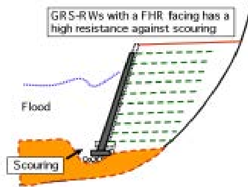
Fig. 11: Good performance of GRS RW with FHR facing in case of scouring [9]
