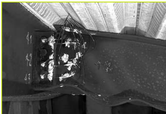
FIGURE 21: Elongation of holes in the beam web in fin plate connection
