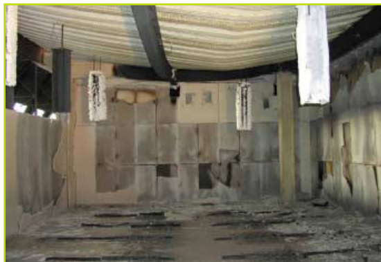
FIGURE 7: Compartment after fire, residual deformation 925 mm, no local collapse of structure
